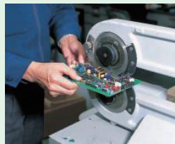
Strain measurement on the process of depaneling
